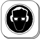
**All persons in the proximity of the machine must wear safety glasses with lateral protection, ear protection as well as safety shoes. The operator is obliged to wear close-fitting protective clothing.**
